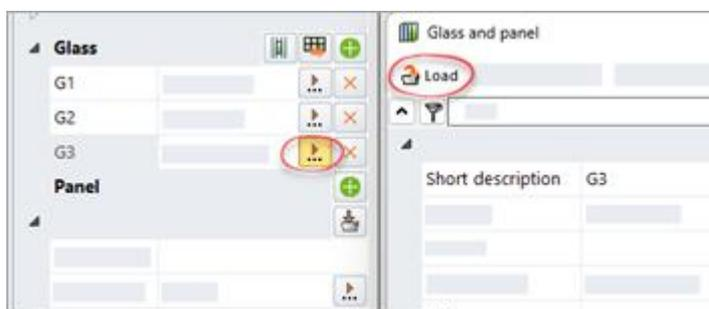
Using the *Load* function, you can change the data for the project glass currently being edited. You can load the data for a glass from the master data or the data for a project glass already in use. Please note the following changes to this function:
